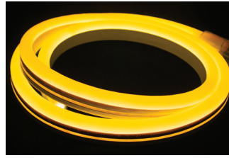
MINI-P2-NF-AY (120V) White LEDs Opaque Amber jacket 590nm • 34Lm/ft
