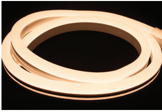
MINI-P2-NF-WW (120V) Warm White LEDs • 79CRI Opaque white jacket 2700K • 90Lm/ft
